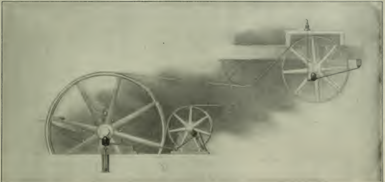
FIG. 1. APPLICATION OF THE RICE ROLLER RELIEF BEARING.
